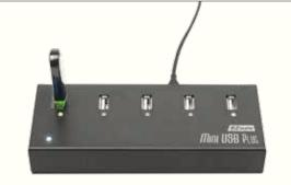
Insert the flash drive with the data to be copied into the Source port. When the green light is on, the machine has detected it. When the green light flashes, it indicates that it starts working.
