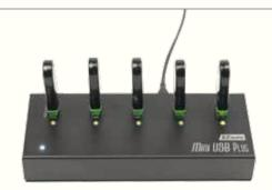
When the green light of the target ports is steady, indicating that the copying process has been completed, you can immediately unplug the copied flash drive and insert the next blank flash drive for copying, without waiting for all the flash drives to complete and then change to the next round.
